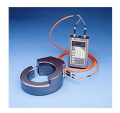
ETS-Lindgren's Model HI-3702 Clamp-on Induced Current Meter measures RF induced body currents using a clamp-on current sensor, sized for a comfortable fit to ankles or arms. This design allows measurements to be taken while walking or climbing. The HI-3702 uses fiber optic technology to eliminate perturbations of the field, and a thermally-based true RMS-DC converter circuit improves measurement accuracy.
