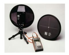
ETS-Lindgren's Model HI-3638 VLF/ELF Electric Field Meter is a EMF meter that has full ELF (extremely low frequency) and VLF (very low frequency) capability to the Swedish MPR and the IEEE 1140 test requirements in a single meter, making electric field testing guick and simple.
