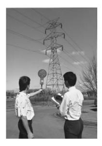
ETS-Lindgren's HI-3604 ELF Survey Meter is a magnetic field probe designed to evaluate both electric and magnetic fields associated with 50/60 Hz power lines, line-powered equipment and appliances. The HI-3604 ELF (extremely low frequency) Survey Meter provides the engineer, industrial hygienist and health and safety professional with a sophisticated piece of surveying equipment for accurate investigation of power frequency environments.
