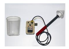
ETS-Lindgren's Model HI-1801 Microwave Oven Survey Meter is a durable, compact and portable insturment for accurately measuring microwave oven radiation. The HI-1801 Microwave Oven Survey Meter is especially suited for appliance service applications, ideal for public health agencies and service technicians to check microwave oven radiation leakage. The CHECK feature on the HI-1801 allows the user to determine that the microwave oven and meter are both operating properly.
