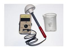
ETS-Lindgren's Model HI-1600 Microwave Meter is a microwave oven survey meter used to measure microwave oven radiation leakage from microwave ovens operating at 2450 MHz or 915 MHz. This survey meter portability for use by microwave oven manufacturers, service technicians, regulatory agencies and public health officials. Three survey ranges are incorporated into a switching sequence that includes positions for battery and probe checks.
