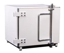
ETS-Lindgren's 5230 Tabletop RF Test Enclosures are cells for conducting sensitive DUT measurements requiring shielding, such as mobile phones. Series 5230 enclosures are produced of welded construction and include doors with progressive RF gasket compression mechanisms, which combined provides RF isolation of up to 120 dB at frequencies above 10 MHz. The large, unobstructed interior and zero perimeter doors maximize the available test volume for larger-sized DUTs.
