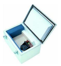
ETS-Lindgren's Model 5211 Wireless Interface Test System (WITS) is a self-contained portable enclosure that can check cell phone transmit and receive functionality with or without direct cable connection to the RF or data ports. This is accomplished using a patent-pending near field coupler in the enclosure that couples with the phone's own antenna. The coupling coefficient has a flat response over the frequency range of 700 MHz to 2 GHz.
