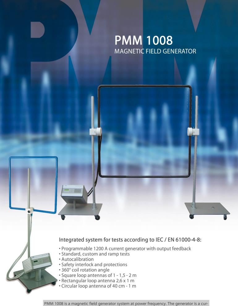
PMM 1008 is a magnetic field generator system at power frequency. The generator is a current generator and the indication of the field is obtained considering the antenna factor, the system includes the antenna formed by one coil and the antenna mast.
