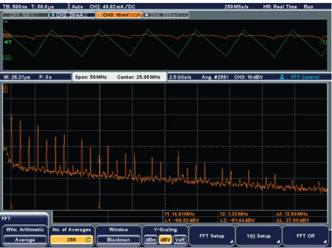
FFT analysis: fast identification of harmonics at the output voltage of a DC/DC converter.
