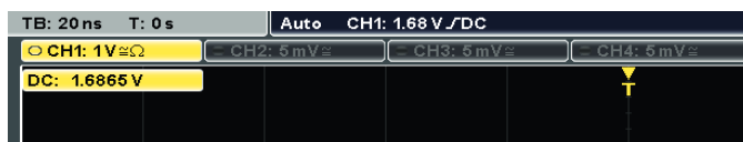
R&S®ProbeMeter: high DC measurement accuracy regardless of instrument settings.
